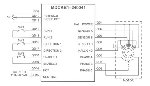
Note: The MDCKB1-240041 driver is not line isolated. Use only mechanical switches for the control inputs. The terminals of motor connector contains high voltage. Do not probe any part of the driver with power on, this could damage the drive or result in body injury.
